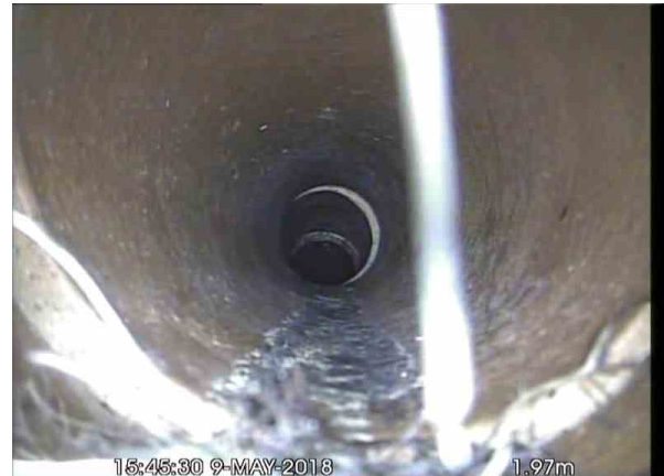
, 00:00:19, 1.97 m General remark, Sewer levels out at this point
